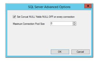
Set Concat NULL Yields NULL OFF This setting allows SQL statements to return data. It can be configured at the session-level or the database level. Because the default configuration at the database level is ON, this box should be checked to override the database-level configuration where SQL statements are to return data. It should only be unchecked if the database has been configured such that Concat NULL Yields is off (for example, to improve performance).
